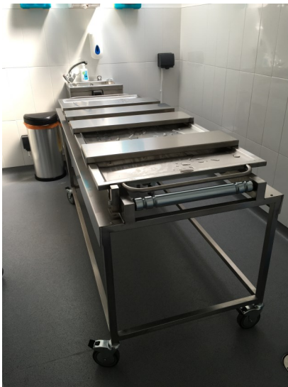
The Roll On / Off mortuary table, reduce lifting and utilise the existing fridge body trays. Transferring the tray from the scissor lifter
